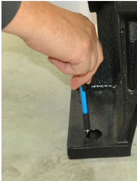
Figure 8a: Mark bore holes
