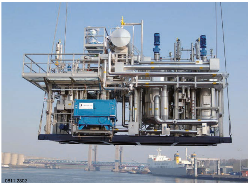
Skid mounted suspension crystallization plant for MDI
