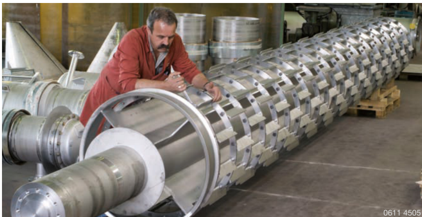
0611 4505 Rotor of a wiped film evaporator
